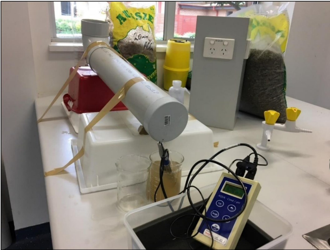
Figure 11. A pilot study that was used to recirculate water through a PVC pipe containing concrete and other aggregate materials. After this pilot study all aggregates were soaked and rinsed in deionised water to remove ‘muddy’ contaminants.
