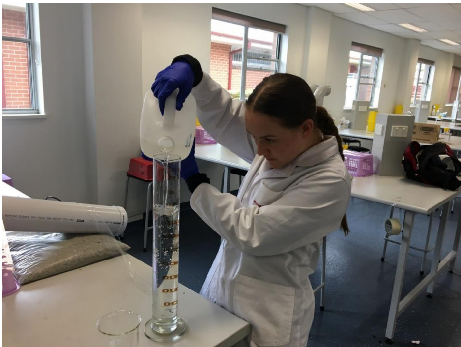
Figure 13. Measuring 1 litre water prior to starting the recirculation experiment. All PVC pipes and laboratory glassware was cleaned and acid-rinsed then deionised water rinsed prior to each recirculation.
