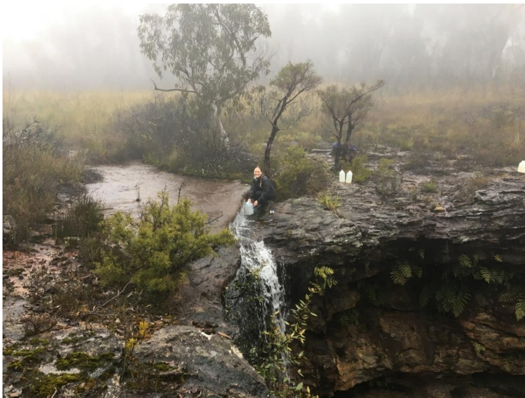
Figure 9. Collecting water that was used in recirculation experiments from the exit stream flowing from the THPSS wetland ‘Mt Hay’ near Leura. The five litre containers were filled with minimal air ‘headspace’ in the containers.
